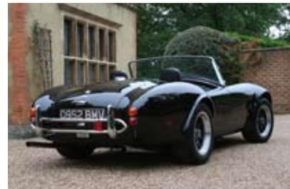
*In 1982, Autokraft managed to get the license to use the name on its own AC Cobra. It differed from the original by its engine, a slightly different bodyline and comfort. The MkIV featured independent suspension, a five-speed Borg-Warner gearbox, a Salisbury limited slip differential and power brakes. Cobra Autokraft are listed in the Shelby Registry, with a total production run of approximately 450 units.*
