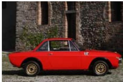
*Pronounce the word "Fanalone" and you will see the eyes of Lancia fans lighting up. It indicates the large headlamps that went on to the final versions of the famous Fulvia 1600 HF, prepared by the plant for its amateur customer drivers. This model also featured a more powerful engine, a new five-speed 'box, a limited slip differential and a light box with extension wings... The car was all ready for rallying, and is now eligible for the most famous of historical events.*
